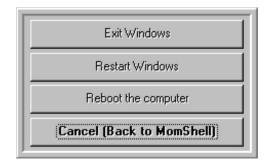
Right clicking the Exit Window button on the Main Window brings the Exit Dialog. You can select to simply Exit Windows (and return to DOS), useful if you are not using MomShell as your Shell, to Restart Windows, or to reboot your computer.
